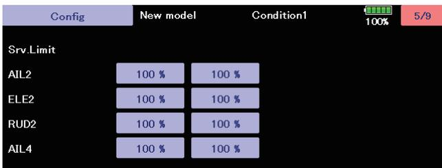
If the SB/R2 port output is set to "S.BUS(HS)" or "S.BUS(STD)", the setting menu will display AIL3 and AIL4 setting items.
