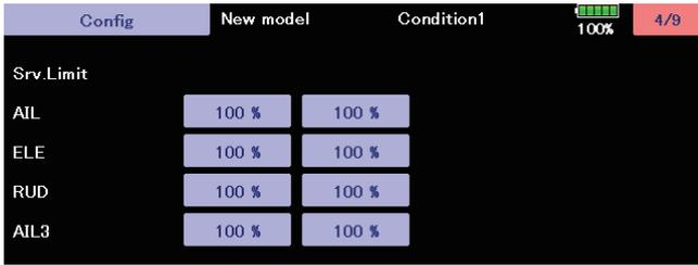
This is the limit setting for each servo. The position of the maximum operation is read into the gyro in the first setting.
