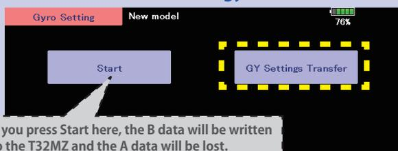
Connect Gyro B to T32MZ and press [GY Settings Transfer]. (Put data on A into gyro B)
