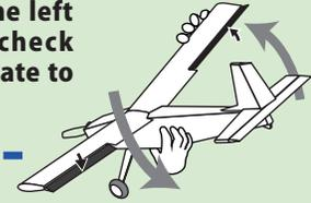
Tilt the airplane to the left on the ground and check that the 4-aileron operate to the right.
