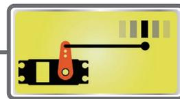
The Sub-Trim function is used to set the servo neutral position, and may be used to make fine adjustments to the control surface after linkages and pushrods are hooked up. When you begin to set up a model, be sure that the digital trims are set to their center position.
