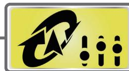
This function is used when a gyro is used to stabilize the fuselage attitude. The sensitivity and operation mode (Normal mode/GYmode) can be switched with a switch.
