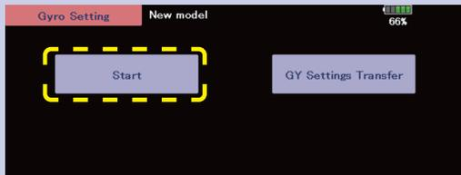
Connect the gyro A to the T32MZ-WC and press [Start]. (Enter the data of A into T32MZ-WC)
