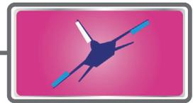
Use this mixing when you want to mix the rudders with aileron operation.
