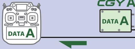
Connect the gyro A to the T32MZ-WC and press [Start]. (Enter the data of A into T32MZ-WC)
