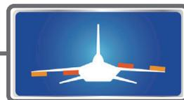
This mixing operates the brake flaps (FLP3/4) in the aileron mode. When the aileron stick is manipulated, the aileron and brake flaps perform the aileron operation simultaneously and the performance of the roll axis is improved.
