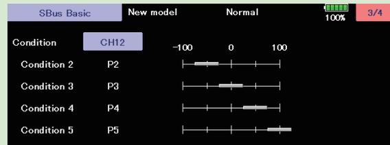
As with the flight condition function of the transmitter, it is possible to utilize pre-determined settings, each activated by a switch or switches on the transmitter. By setting the condition switch on the channel with the AFR function of the transmitter and setting the point for each flight condition with the AFR point curve, you can switch the condition of CGY760R/CGY755 in conjunction with the flight condition switch of the transmitter.
