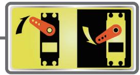
Servo Reverse changes the direction of an individual servo's response to a control stick movement.
