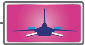
This mixing is used when you want to mix the elevators with airbrake (spoiler) operation. It raises the elevators to correct for drooping of the nose during airbrake operation.
