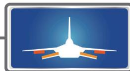
This function is used when you want to mix the camber flaps with elevator operation. When mixing is used so that the flaps are lowered by up elevator, lift can be increased.
