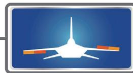
This mixing operates the camber flaps (FLP1/2) in the aileron mode. When the aileron stick is manipulated, the ailerons and camber flaps move simultaneously and the roll axis is improved.
