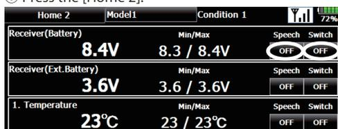
⑦ Speech ON/OFF can be switched by switch. When the [Switch] button is touched the switch setting screen opens. When the set switch is operated voice reading starts. When multiple switches were set to ON simultaneously, setting of the top line has priority.
