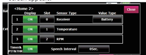
Alternatively, the detail display screen may be accessed as follows: [Linkage Menu] → [Telemetry] → selected sensor → Home 2 [Select]
