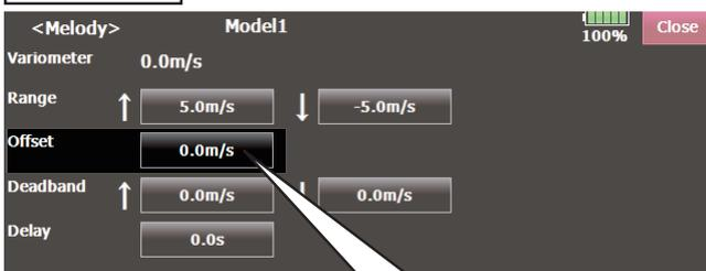
This is the changing point of climb and sink. When the variometer is greater than this value, Vario Melody is climb type. When the variometer is less than this value, Vario Melody is sink type.
