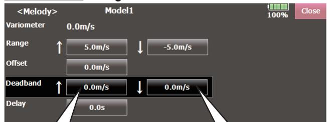
When the variometer is less than this value, Vario melody is not output.
