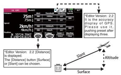
■ GPS (altitude) and GPS (variometer) setting screen This screen displays the altitude, variometer, and air pressure. When [Preset] of [Reference Point (Altitude)] is touched, the altitude measurement reference altitude is initialized
