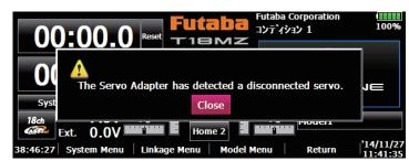
This screen appears and an alarm sounds to indicate a servo connection error.
