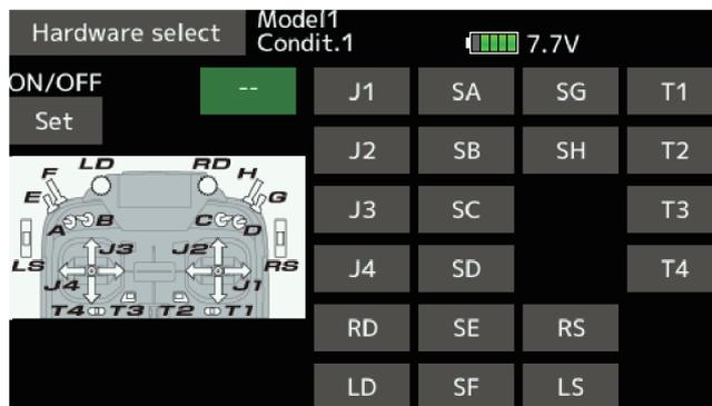
⑤ The operated switch is selected. Sets the current switch position to **ON**. Operating the switch changes the **ON** position.
