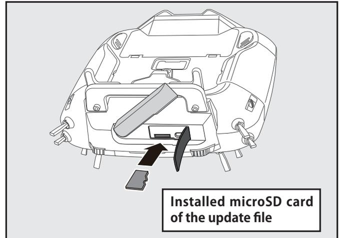
6. Turn on the transmitter power while pressing down the "HOME/EXIT" button. The update screen appears on the LCD display of your T16IZ SUPER and the software update is started.
