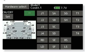
⑤ The operated switch is selected. Sets the current switch position to **ON**. Operating the switch changes the **ON** position.
