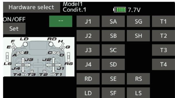
⑤ The operated switch is selected. Sets the current switch position to **ON**. Operating the switch changes the **ON** position.
