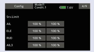
This is the limit setting for each servo. The position of the maximum operation is read into the gyro in the first setting.
