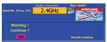
When the throttle stick is returned to the low side, the warning display goes off.
