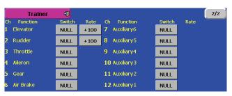
Set the trainer mode to either MIX or FUNC mode. The rate buttons appear on the 2nd page of the trainer screen. Set the student rate as desired.
