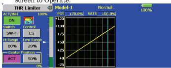
2. When the "Center position" rate is changed, the limit value at the operation hardware neutral position can be adjusted.
