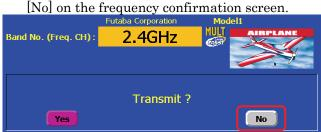
For safety, the RANGE CHECK mode can not be selected while the RF transmission is active.
