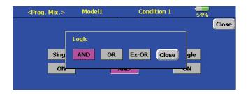
5. The left and right side of the switch mode can be set to the logic switch mode as well. In this case, a maximum of 4 switches can be assigned to the logic switch. The left and right logic are calculated first, then the center of the logic is calculated. Finally, switch on/off status determined by the 4 switches' combination.
