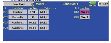
2. The logic switches can be assigned by changing the mode to "Logic" by pressing the "Single" button.
