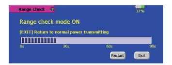
Please note, upon expiration of the 90 seconds, or when [Exit] is selected, the transmitter will automatically return to the normal RF operation as noted on the display.
