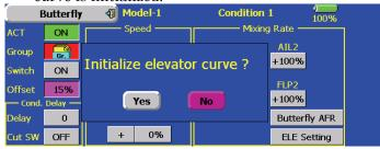
When the ELE setting screen is opened, the curve is initialized.
