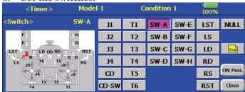
4. Switch the condition and set the switch of each condition.
