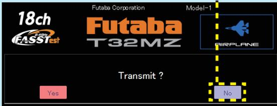
\*For safety reasons, receiver settings cannot be made while radio waves are being transmitted.
