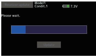
14. The GREEN LED on the R7201SB/R7301SB lights up when the update is complete.
