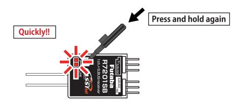
7. Release the switch when the solid orange.
