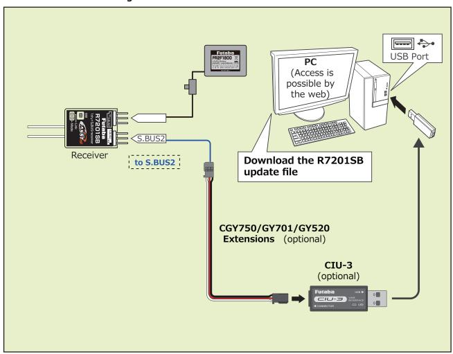
4. Turn on the receiver power while pressing down the switch.
