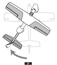
Tilt the airplane to the left on the ground and check that the ailerons operate to the right.  $\sqrt{2}$
