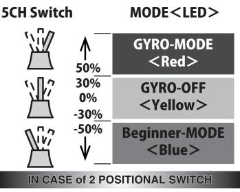
When there are no 3-position switch in a transmitter.
