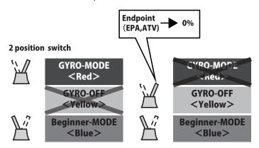
In the case of a beginner, the side at which the CH5 end point (EPA, ATV) switch is pushed forward should be made 0% and the mode should be switched between the GYRO OFF mode and Beginner mode.
