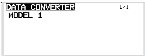
3. The converter shows a list of model data in the card. Select a model data that you want to convert and push "RTN" key, and the converter should begin converting data.
