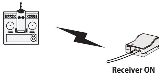
8. If linking fails, an error message is displayed. Bring the transmitter closer to the receiver and repeat the procedure above from Step 2.
