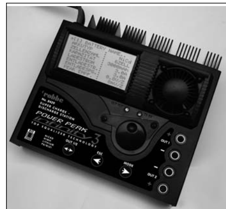
Power Peak Infinity 3 No. 8429 The ultimate intelligent home charging station incorporating convenient battery management. For charging and discharg- ing NC, NiMH, Lead and Lithium batteries. Cell counts NC batteries: 1 ... 30 cells NiMH batteries: 1 ... 30 cells Lead-acid batteries: 1 ... 6 cells Lithium batteries: 1 ... 12 cells Charge / discharge current 0.1 ... 10 A
