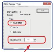
When MAGNETIC type is selected, GEAR RATIO is needed.
