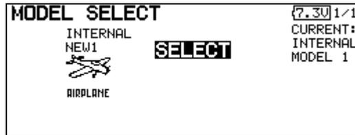
4.4. The message of confirming is displayed. Please push the dial. So the model is changed. The model data is recovered automatically.
