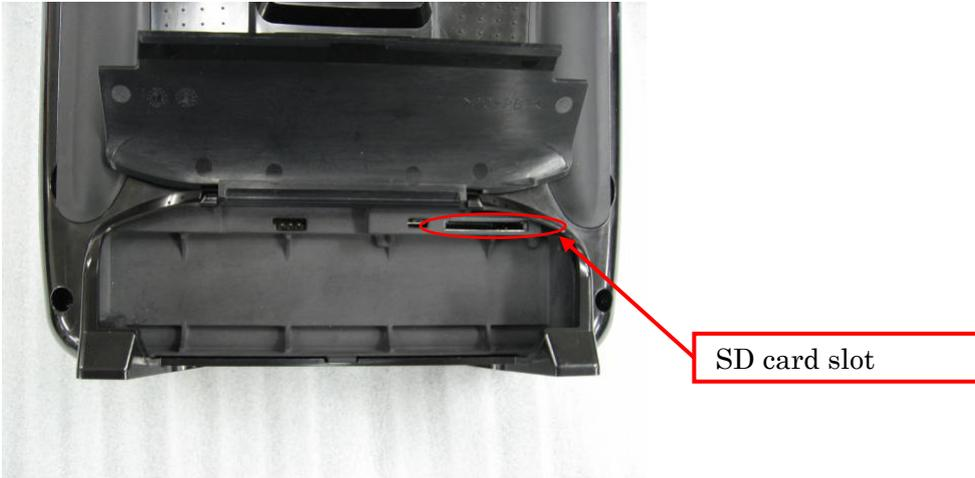
1.2. Please turn on power switch of T12FG. If the SD card not formatted is set, the following screen is displayed. Please rotate the dial of T12FG, select "Format" and push the dial.
