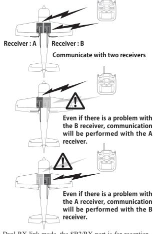
In Dual RX link mode, the SB2/RX port is for reception only, so use CH mode B, C, D, F, G mode for S.BUS output and S.BUS2 input/output.
