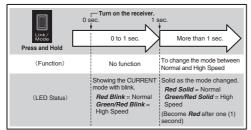
Please check the operation mode by observing the **LED** when turning on the receiver. If possible there's no **FASST** transmitter turned on around you in order to make firmer check.
