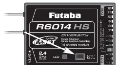
This permanent assignment between transmitter and receiver provides a superb basis for suppression of interference signals. Suppression is even better than that of conventional systems, since a digital filter is used to allow through only those control signals which emanate from the receiver’s bound transmitter. The net result is extremely effective suppression of interference and signals from other transmitters.
