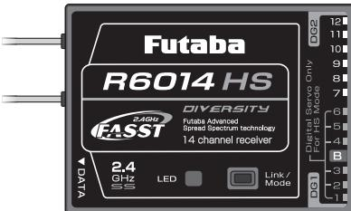
The R 6014HS receiver features a select switch for digital and analogue servos. This makes it possible for the signals to be passed to digital servos connected to outputs 1 - 6 at a higher rate, resulting in even faster servo response. With dual-aerial diversity system. A jumper is fitted which allows channels 11 + 12 to be used with the MPDX1 Multi-prop decoder, expanding each channel to eight multi-prop channels.
