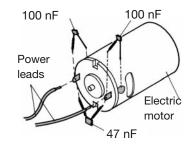
No. 4008. Each motor must be suppressed individually, as shown in the drawing.
