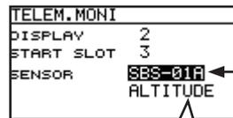
When using a sensor that has two or more functions, you will want to scroll to select which will be displayed. (ALTITUDE,VARIO, etc.)
