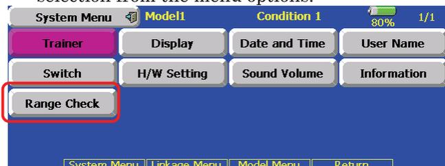
3. The Range Check screen is displayed. To activate the Range Check mode press the [Yes] button. During the Range Check period, the RF power is reduced to allow the ground range tests to be performed.
